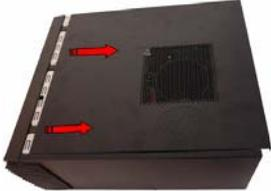
A black PC case with a sliding side cover. Red arrows indicate the cover sliding back and being lifted. |
