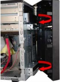
A photograph showing the front panel being reattached to the server chassis. Two red curved arrows indicate the downward and inward movement of the panel.                |
