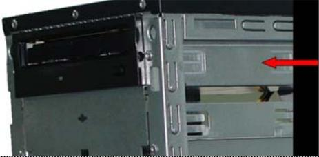
A close-up photograph of the optical drive bay. A red arrow points to the screws on the right side of the drive's front panel that are being removed.                       |
