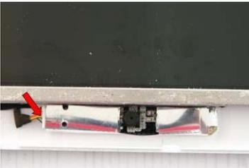
A close-up photograph of the webcam assembly. A red arrow points to a small connector on the left side of the assembly.                    |
