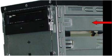
A close-up photograph of the drive tray. A red arrow points to the screws that hold the tray in place.                                                            |
