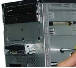
A close-up photograph of a screwdriver being used to remove screws from the front of a floppy disk drive mounted in a server rack.                                         |
