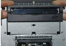
A photograph showing a hand inserting a new optical drive into the tray. The drive is being pushed into the tray.                                               |
