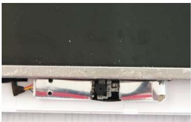
A close-up photograph of the webcam assembly, showing the new camera module installed in place of the old one.                            |
