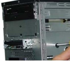
A close-up photograph of a screwdriver being used to install screws into the front of a floppy disk drive.                                                                |
