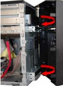
A photograph showing the front panel being reattached to the drive bay. Red curved arrows indicate the downward and inward movement of the panel.              |
