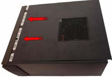
A photograph of a black computer tower case. Two red arrows point to the screws on the left side panel, indicating where to attach it.                                                                                                                        |
