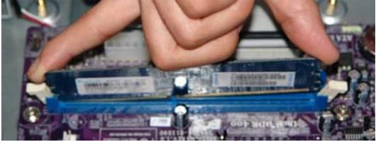
A hand inserting a blue RAM module into a slot on a motherboard, ensuring it is properly seated.        |
