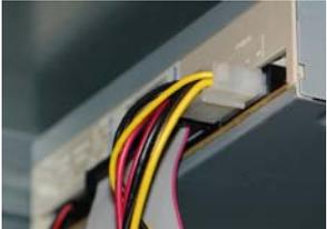
A close-up photograph of the back of the optical drive. Several colored cables (yellow, red, blue, black) are being plugged into the drive's connectors.        |
