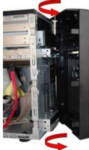
A photograph showing the front panel of a drive bay being lifted away from the chassis. Red curved arrows indicate the upward and outward movement of the panel. |
