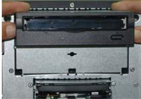
A photograph showing a hand pulling the optical drive out of the tray. The drive is being moved towards the front of the tray.                                   |
