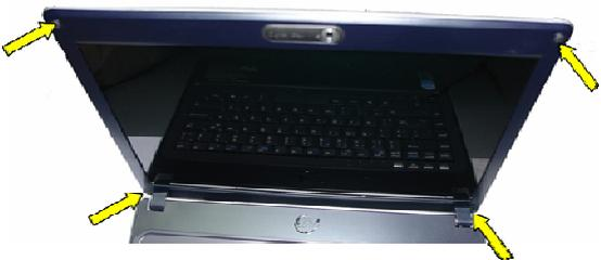
A photograph of the blue laptop with its screen open, showing the screws at the corners of the screen bezel highlighted by yellow arrows. |
