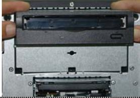
A photograph showing the optical drive being pulled out of its bay. The drive is shown partially extended from the chassis.                                                |
