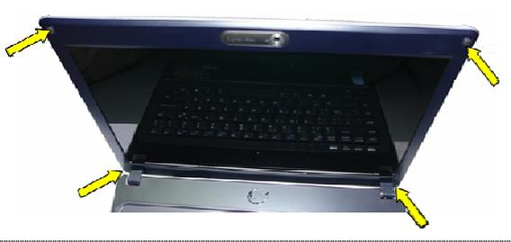
A photograph of a blue laptop with its screen open. Four yellow arrows point to the screws located at the corners of the screen bezel, which hold the plastic cover in place.                        |
