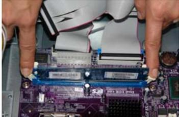
A hand pressing down on the retention clips of a blue RAM module on a motherboard.                      |
