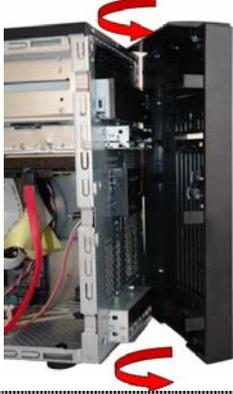
A photograph showing the front panel of a server chassis being lifted away from the main unit. Two red curved arrows indicate the upward and outward movement of the panel. |
