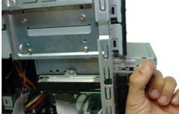
A photograph showing a hand sliding the floppy disk drive out of its metal housing in the server chassis.                                                             |
