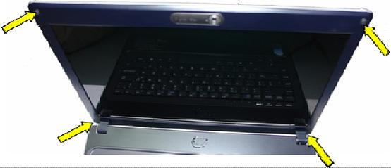
A photograph of a blue laptop with its screen open. Four yellow arrows point to the screws located at the corners of the screen bezel.      |
