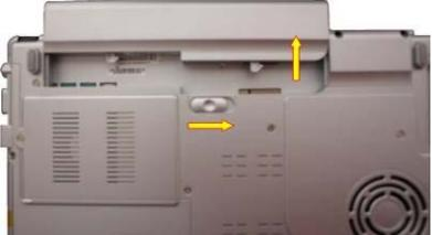
A photograph of the rear panel of the device with a yellow arrow pointing to a small button on the battery cover and another yellow arrow pointing to the right, indicating the direction to slide the cover. |
