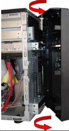
A photograph showing the front panel of a server rack being lifted away from the chassis. Two red curved arrows indicate the upward and outward movement of the panel. |
