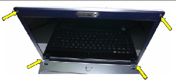
A photograph of the blue laptop with its screen open. Four yellow arrows point to the screws at the corners of the screen bezel, indicating they are being reinserted to secure the plastic cover. |
