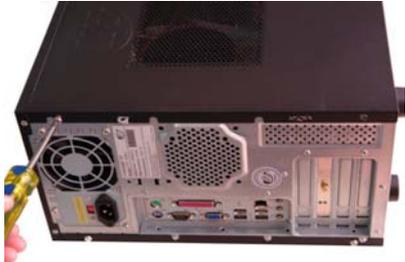
A hand using a yellow and blue screwdriver to remove a screw from the back of a black PC case.           |
